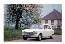
In 1965, Peugeot launched the 204 with a body designed by Pininfarina and front wheel drive with a light alloy engine and an integral transmission lubricated by the same oil as the engine.
