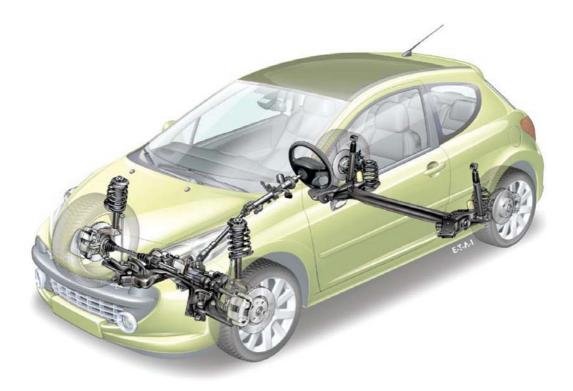
Like all 207s, the front suspension consists of a pseudo McPherson type strut assembly and for the rear suspension a torsion beam. This design ensures both low weight and compact overall dimensions, whilst still ensuring considerable rigidity, which reduces noise and ensures good body control.
