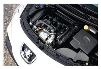
The EP6DT engine used in the 207 GT has a sixteen valve cylinder head with two overhead camshafts and 4 cylinders displacing 1598cc. It produces a maximum power output of 110kW at 5800rpm.
