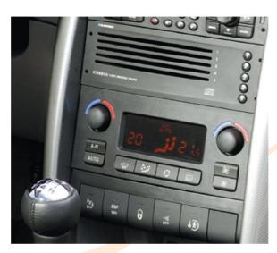
A "Dual-zone" air conditioning with climate control system is fitted as standard on the XE and GT models. It allows the driver and front passenger to control their temperature and airflow distribution independently. It is combined with a sun sensor located on the fascia panel which anticipates the effects of a period of intense exposure to the sun or, conversely, the passing through of a tunnel, in order to temporarily correct the reference temperature level.
